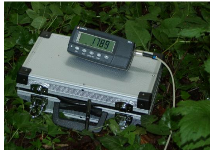
Force sensor and force display
