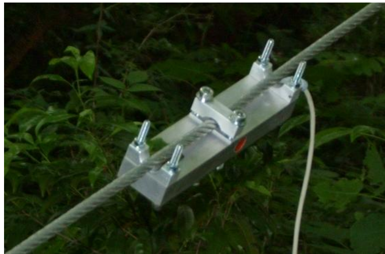
Force sensor and force display
