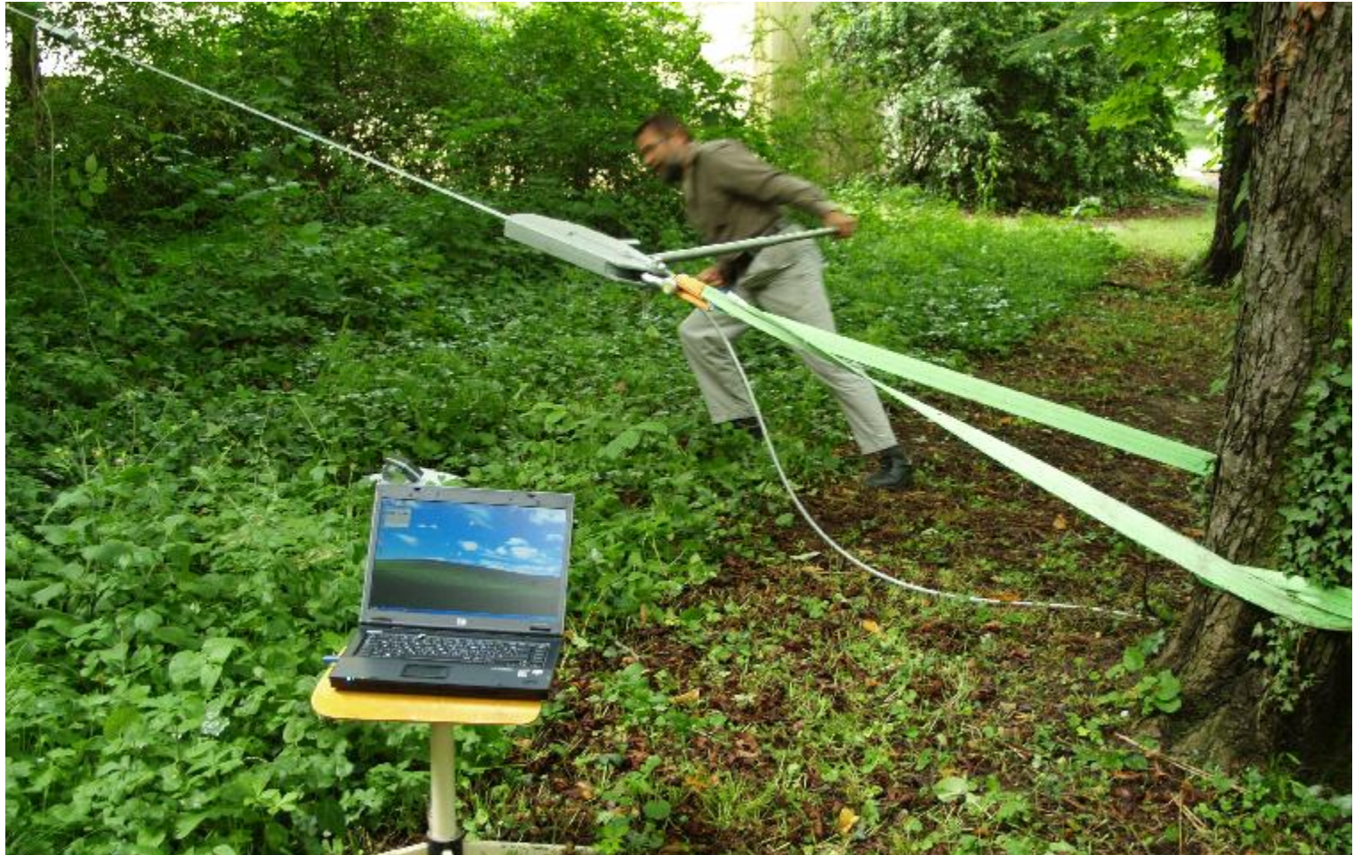
Pulling test is in progress in Hungary.
